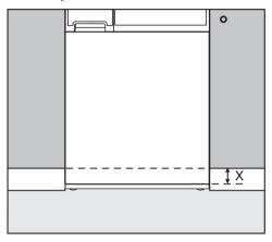
The measure **X** equals the space from the bottom of the washer door to the bottom of the adjacent cabinet.
